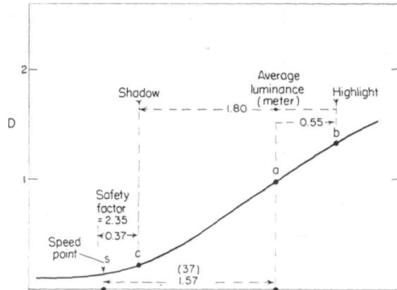
camera image of an average exterior scene when the camera exposure is based on the ASA exposure index and the exposure-meter reading of the average luminance of the scene.
