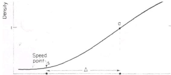
Fig. 2. The D-log E curve for a negative film, showing the location of the exposure,  $E_a$ , for the gray object measured by the exposure meter.
