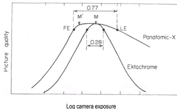
Fig. 11. The picture-quality vs. log-camera-exposure curve for the black-and-white film compared with the corresponding curve for the color reversal film having the same exposure index. FE represents "first excellent," LE, "last excellent." M represents the present exposure level; M', the proposed exposure level for the black-and-white film.
