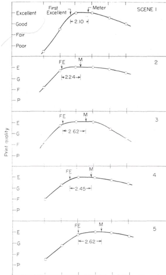
Fig. 5. The print-quality vs. log-camera-exposure curves obtained by the experimental method. The number shown under each curve is the safety factor.
