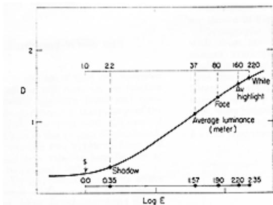
Fig. 8. The exposure levels, for various scene elements, associated with the safety factor of 2.4.
