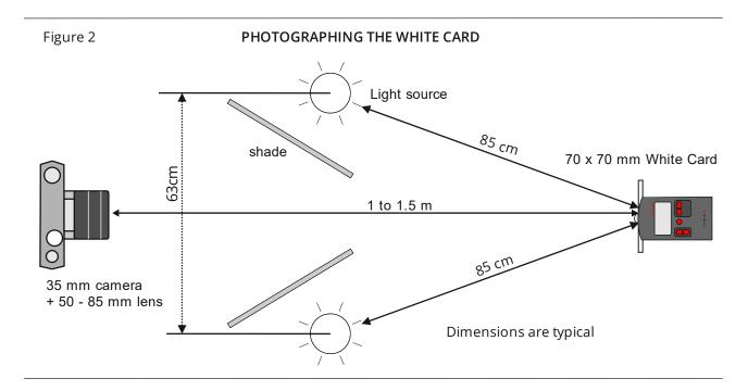
Two exposures are made of the white card representing H2 as the normal exposure reference and H4 where the difference is 62/3 stops.
